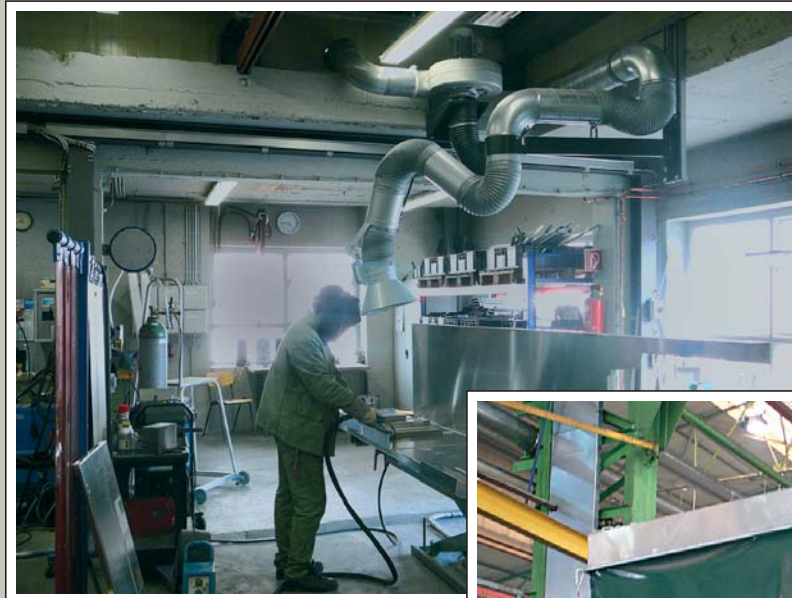
Aluminium work base with an extreme flexible and light moveable extraction arm in 200ø – 3m long.
