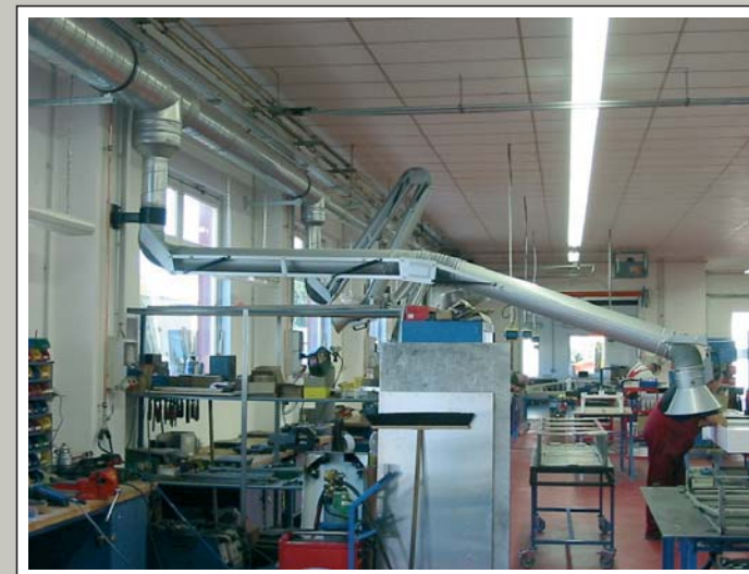
Extraction Arms 160ø – 4 m long with wall brackets for welding extraction as a central pipe and filtration system for industrial use.
