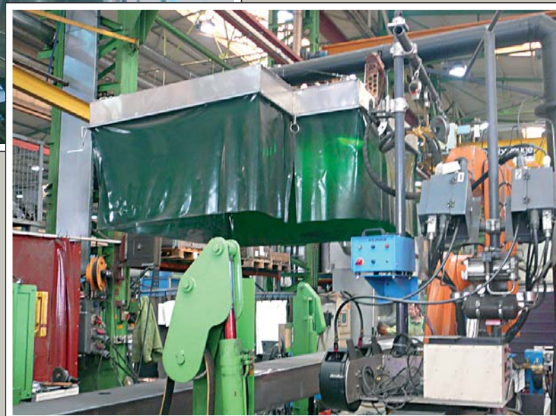
Pivoting and moveable Suction Hood for robotic welding work bases with SSK 290 and a central cartridge Filtration.
