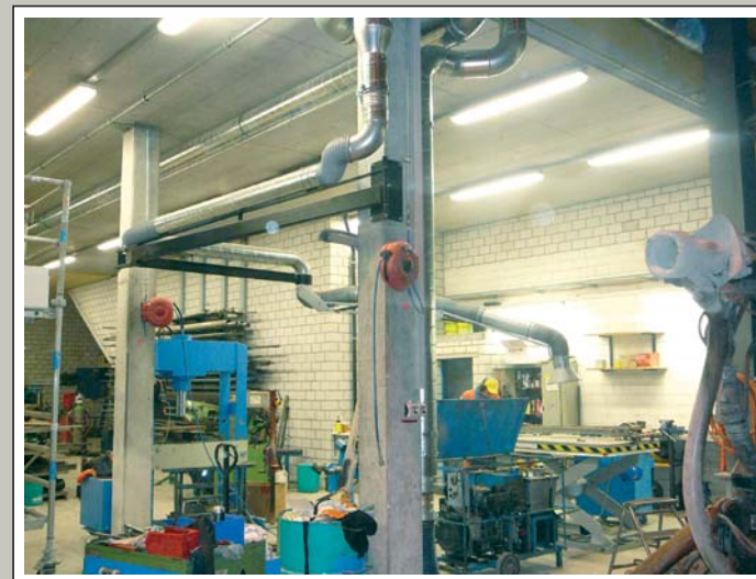
Very flexible VARIO Flex Arm 160ø – 9 m long, with 3 swivelling points, mounted on a column for 4 workplaces.
