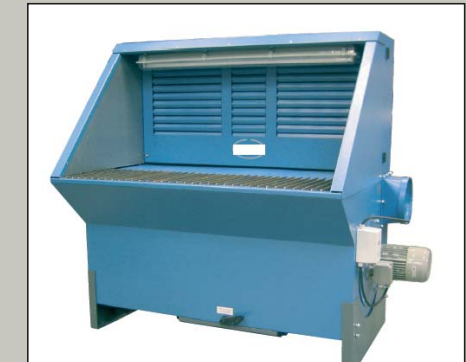
Grinding/Sanding table with under and back plate extraction by the integrated fan and cartridge filter for the operation with circulating air
