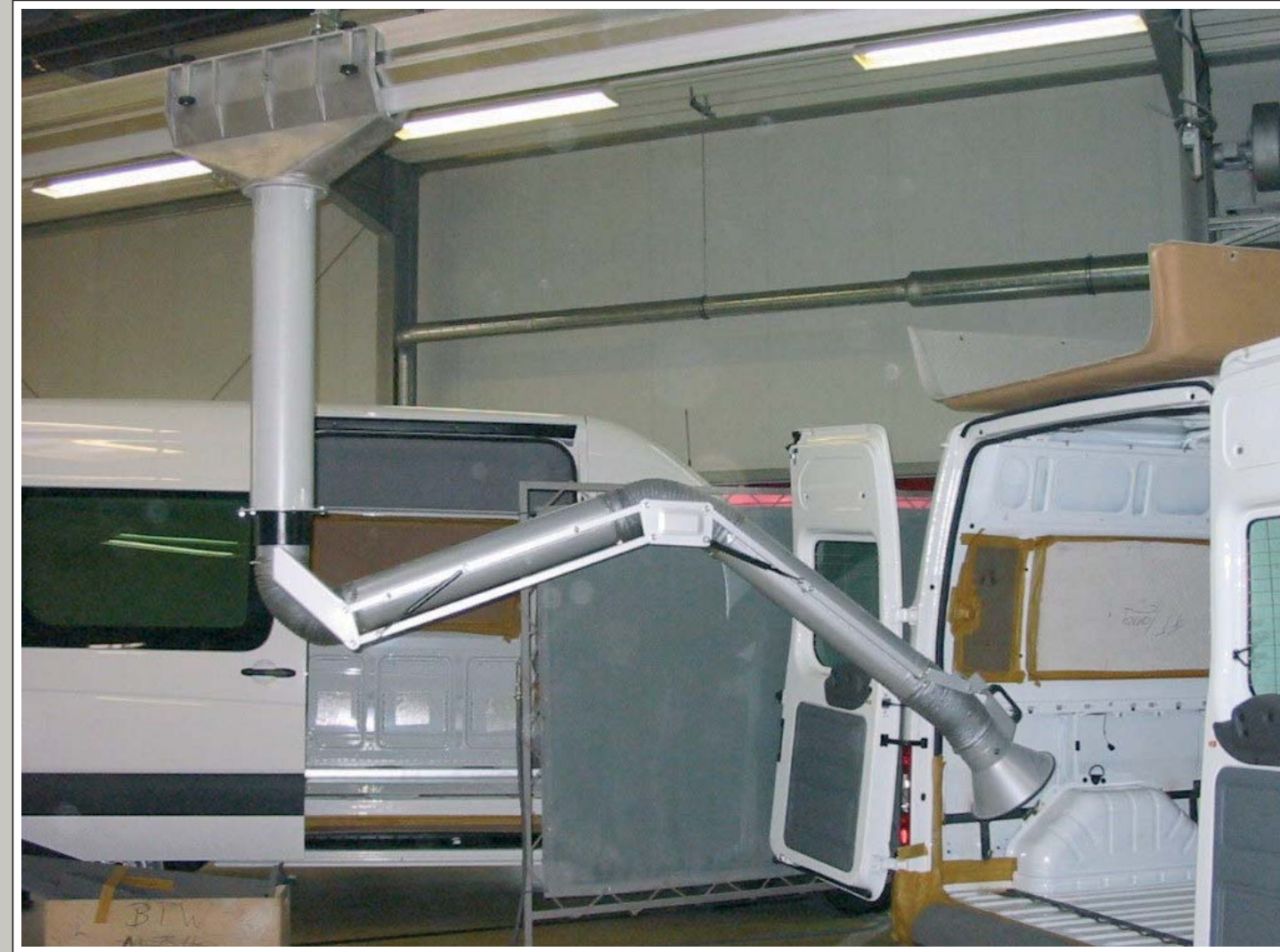
Big Trolley in aluminium rail system type SSK 290 with a lengthening pipe and suction arm 160ø for welding extraction.
