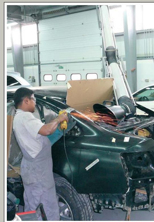
Suction of sparking and fine dust during repairing of body parts on a car.
