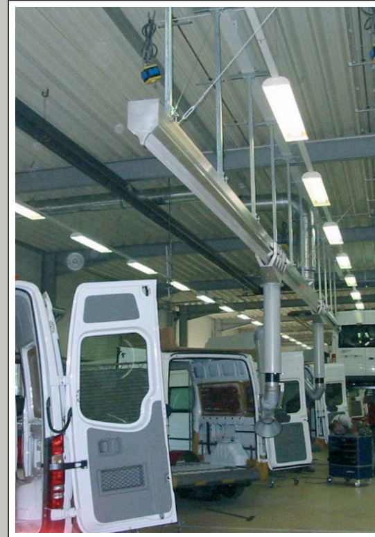
Aluminium rail system type SSK 290 with moving extraction arms for welding in a body workshop of transporter cars.
