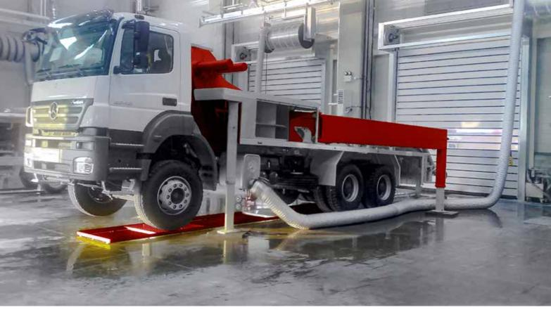
To guarantee the optimum capture of harmful substances from diesel engine emissions for agricultural machines and construction machines, the exhaust gas flow of the test vehicle should be taken into account. The key parameters are the cubic capacity and the rpm of the engine along with the combustion process (spark ignition or self-ignition).
