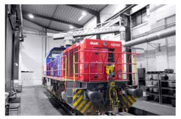
**Swivel-mounted aluminium rail system** – The swivel-aluminium rail system is a fixed solution for capturing harmful substances from diesel motor emissions within a larger radius of 3-9 m. The bracket can be fully rotated more than  $180^{\circ}$  and the carriages are controlled along the rails either manually or electrically. The extractor hood can also be lowered onto the exhaust either mechanically or electrically.
