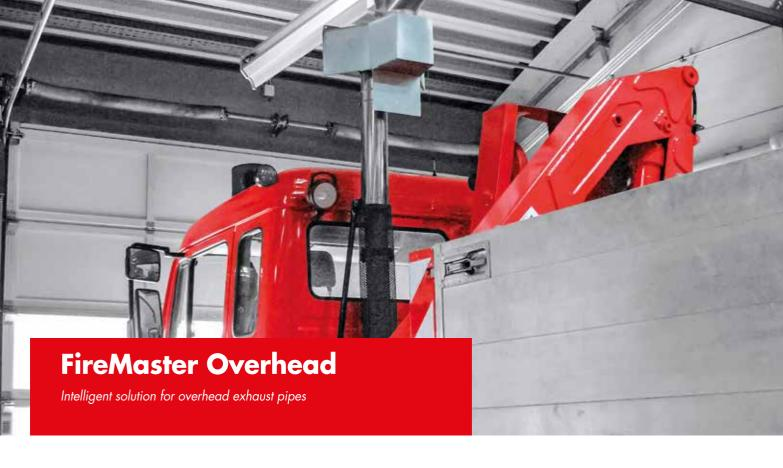
The FireMaster Overhead system was developed for targeted, efficient detection of exhaust gases from vehicles with overhead exhaust pipes. The overhead system consists of a suction slot channel with carriage and a suction hood which is automatically coupled via magnets on the vehicle. The magnet (anchor plate) is attached to the exhaust tailpipe of the emergency vehicle.
