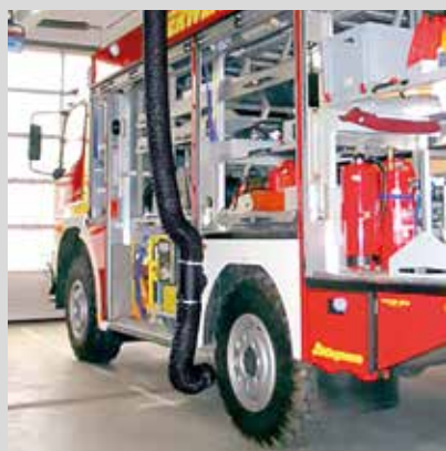
The magnetic coupling can be flexibly mounted depending on the vehicle.
