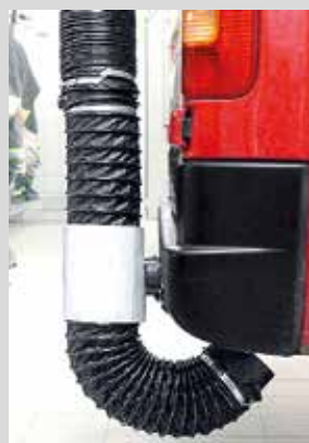
The magnetic coupling can be flexibly mounted depending on the vehicle.
