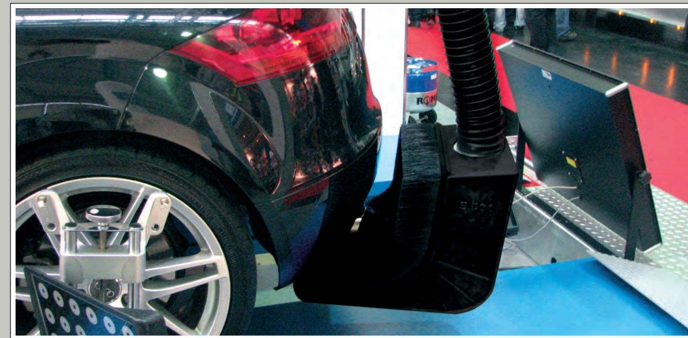
New capture element from type SLS-Car by usage at a measurement work bay in Audi workshop.
