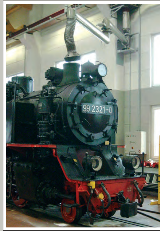
Steam locomotive extraction at Molln in Bad Doberan via multiple joint extraction arm with \varnothing 200 and a max. reach of 5 m, with custom design for exhaust gases containing extreme amounts of sulphuric acid.
