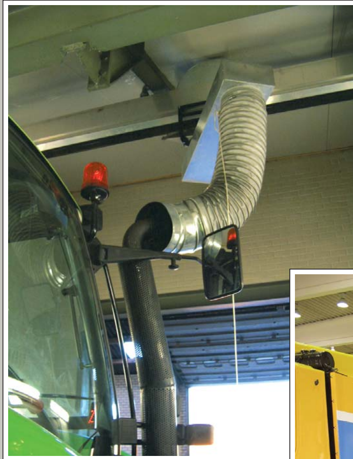
High temperature – Extraction unit for performance test / dyno test.
