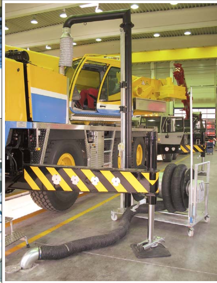
Mobile extraction hose reel (on carriage) for overhead high exhaust systems. Easy attachment on existing under floor extraction system.
