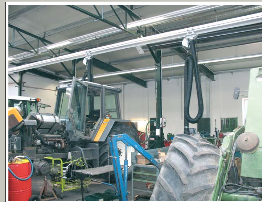
Rail system SSK 290 with 2 hose trolley units for nominal diameter 100 mm.
