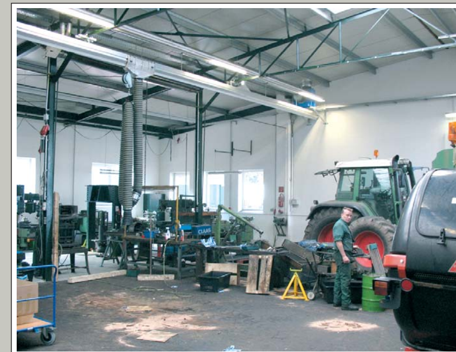
Rail system SSK 290 with hose trolley for nominal diameter 200 mm.
