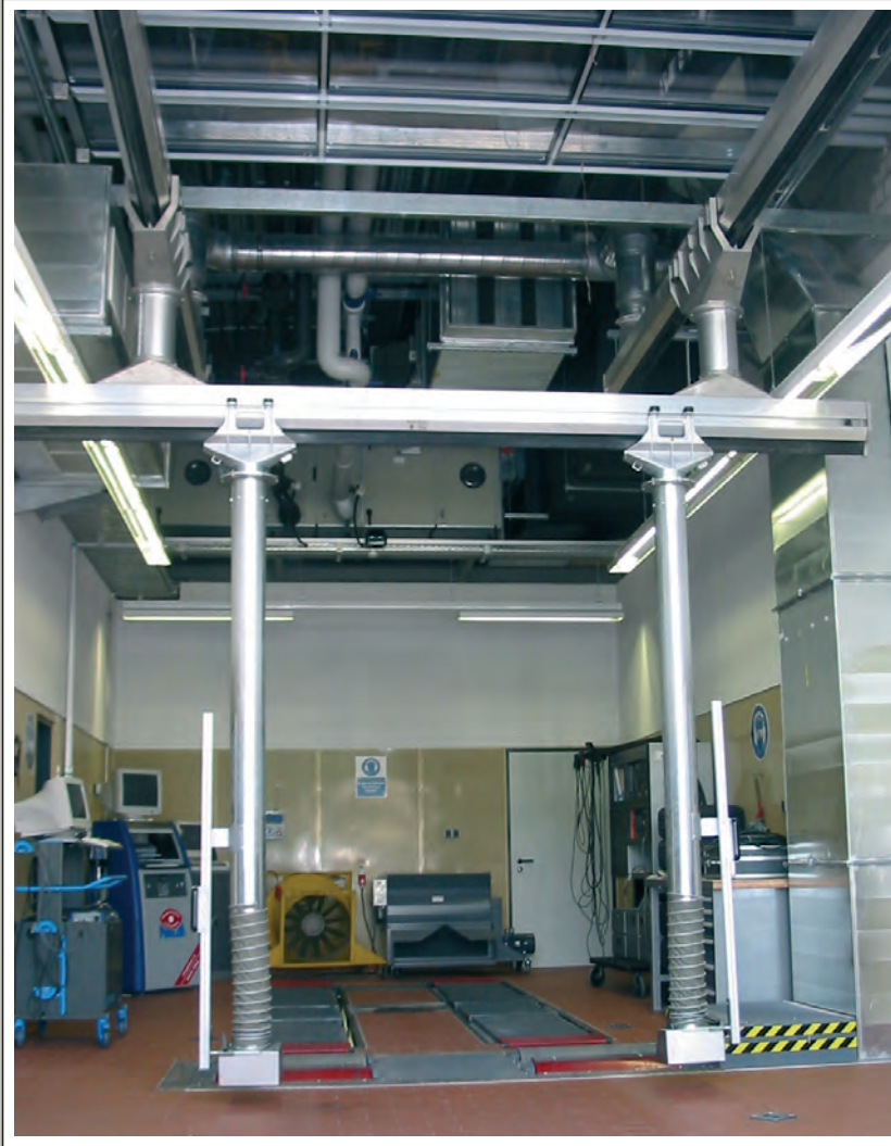
Rail system SSK 290 as movable coordinate system for passenger car performance test beds with suction performance of up to 4,000 m 3 /h and available as high temperature version for exhaust gas temperatures of up to 900°C.
